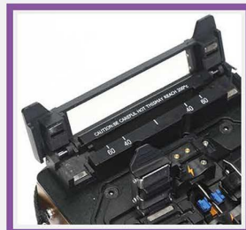
Fast heating, temperature can reach 250 °C
